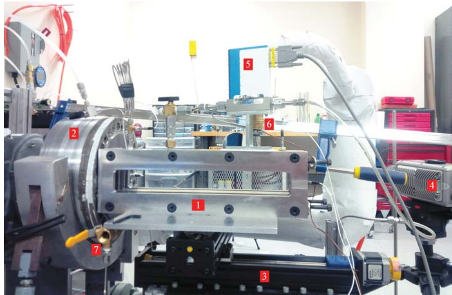
Fig. 2.1.: Combustion chamber (1) sitting on XY positioning table (3) while facing the pre-chamber (2). A C-clamp (6) holds it firmly in place. Also shown are air inlet (6) and outlet (7) for main chamber heating and mass flow controller (5) for fuel delivery and a High speed camera (4).
