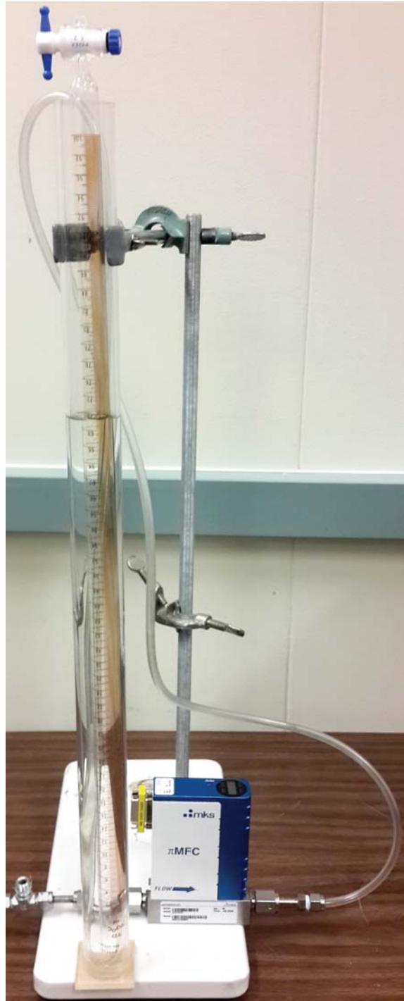
Fig. 2.17.: Volume displacement set up used for calibrating the MFC
